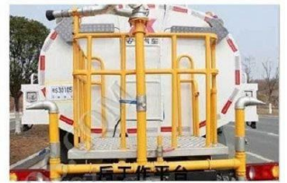
Back Working Platform
